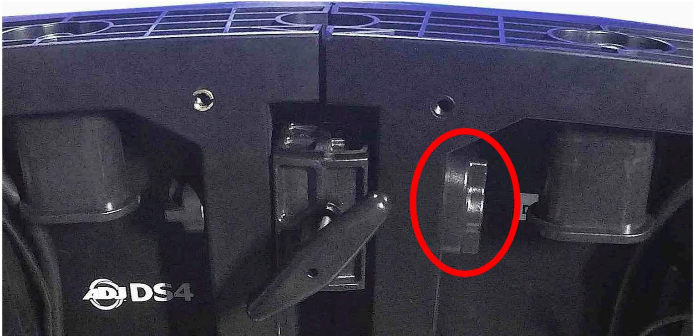
1. With the DS4CC Curve Connectors installed in both panels, twist their locking mechanism knobs 90° to lock them in place.
