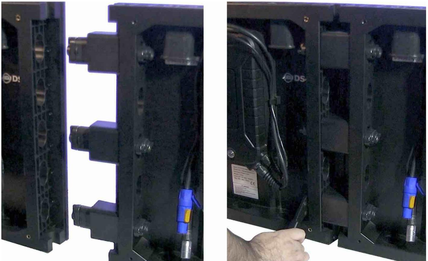
With the DS4HC Horizontal Connectors installed in both panels, twist their locking mechanism knobs 90° to lock them in place.
