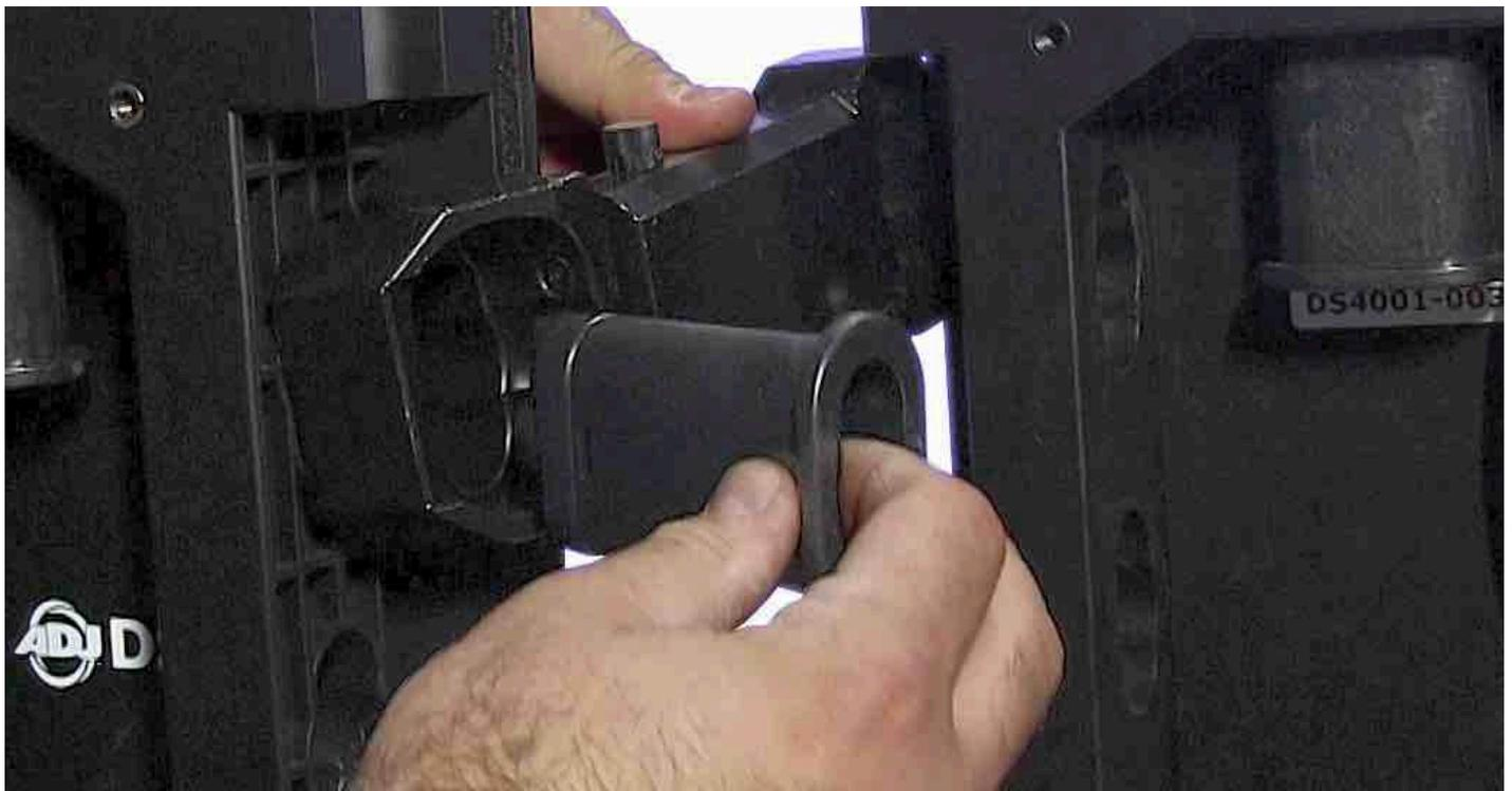
1. Secure the DS4OB Offset Bar to the panel with a DS4VC Vertical Connector.
