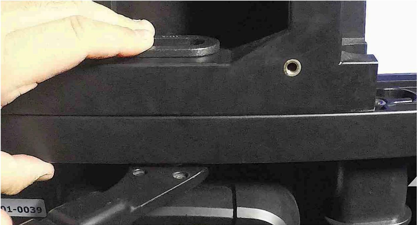
1. Use the DS4FW Fastening Wrench to turn the more difficult to reach, or hard to turn locking mechanism knobs.
