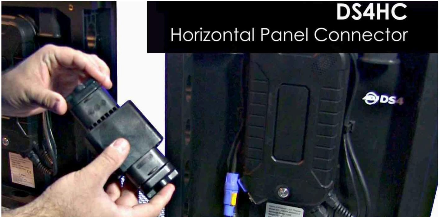
The DS4HC Horizontal Connectors have panel locking mechanisms on both sides with a panel spacer sleeve between them.
