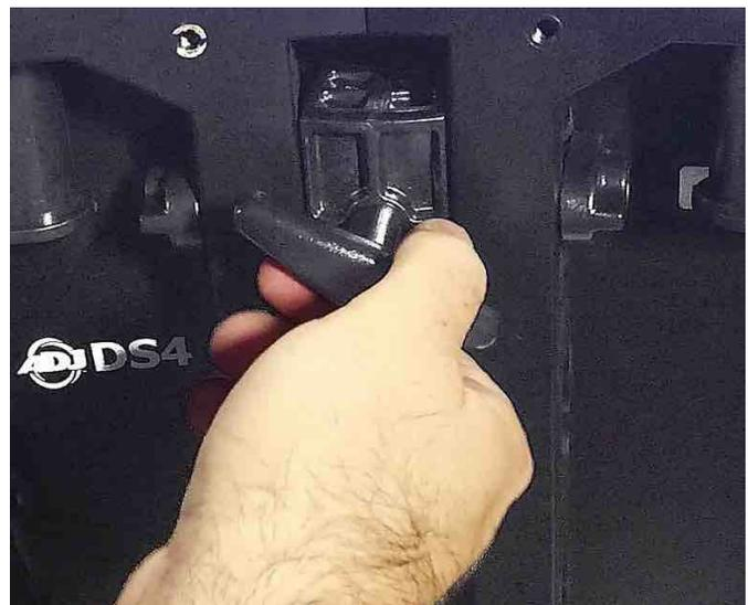
3. Twist the angle lock to secure the desired panel angle position
