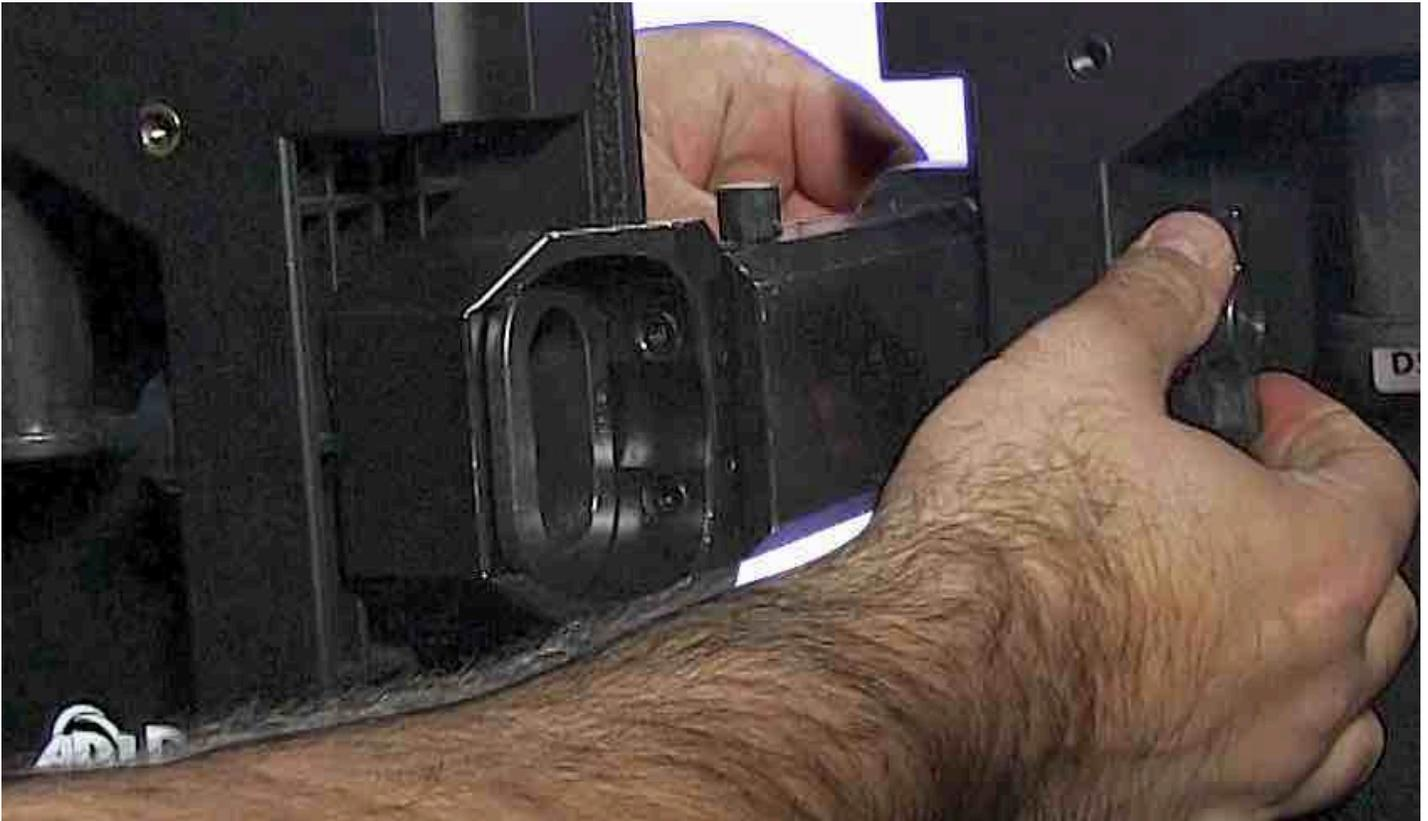
3. With the DS4OB Offset Bars in position, and the second set of DS4HC Horizontal Connectors installed, twist their locking mechanism knobs 90° to lock them in place.
