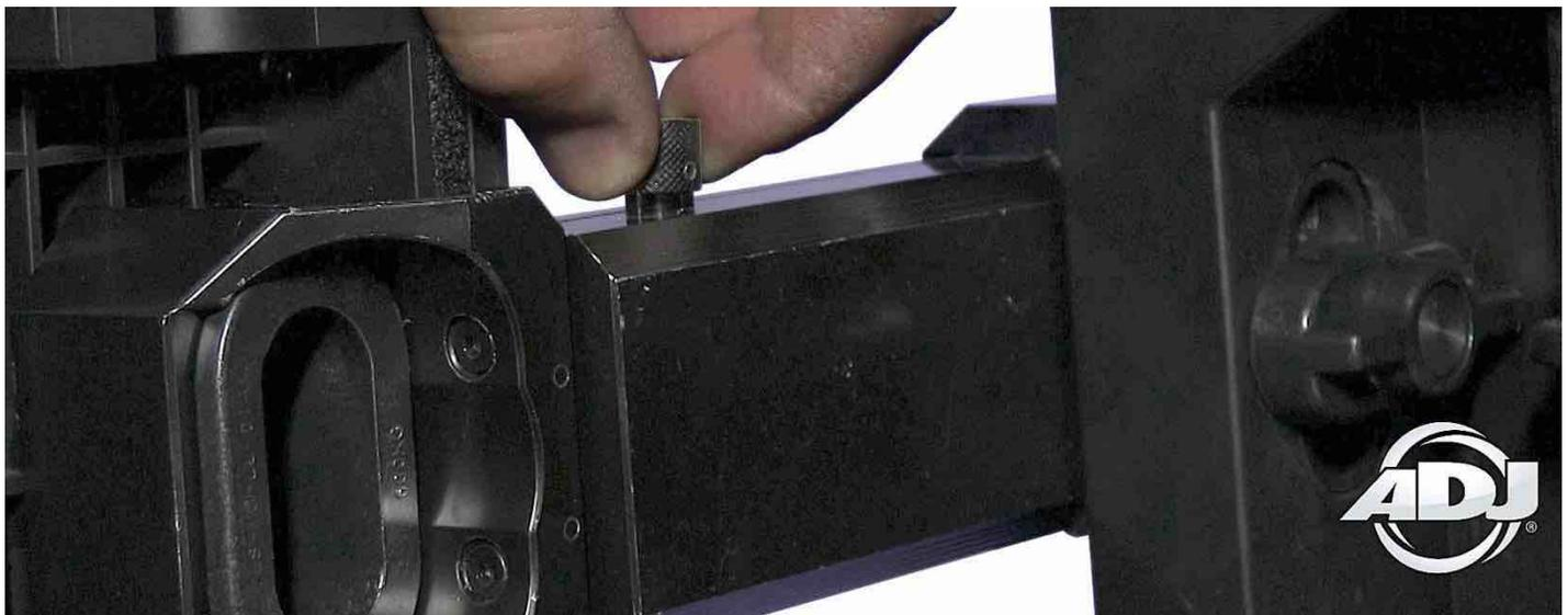
5. Pull and twist the knurled spring-loaded locking pin to an open position on the DS4OB Offset Bar, extend the panel, then re-engage the locking pin.
