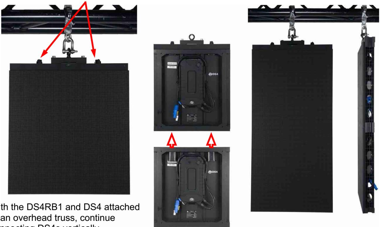
3. With the DS4RB1 and DS4 attached to an overhead truss, continue connecting DS4s vertically.
