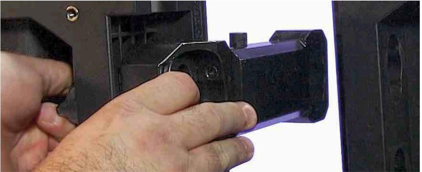
2. Twist the locking mechanism knobs of the DS4VC Vertical Connectors 90° to lock them in place.
