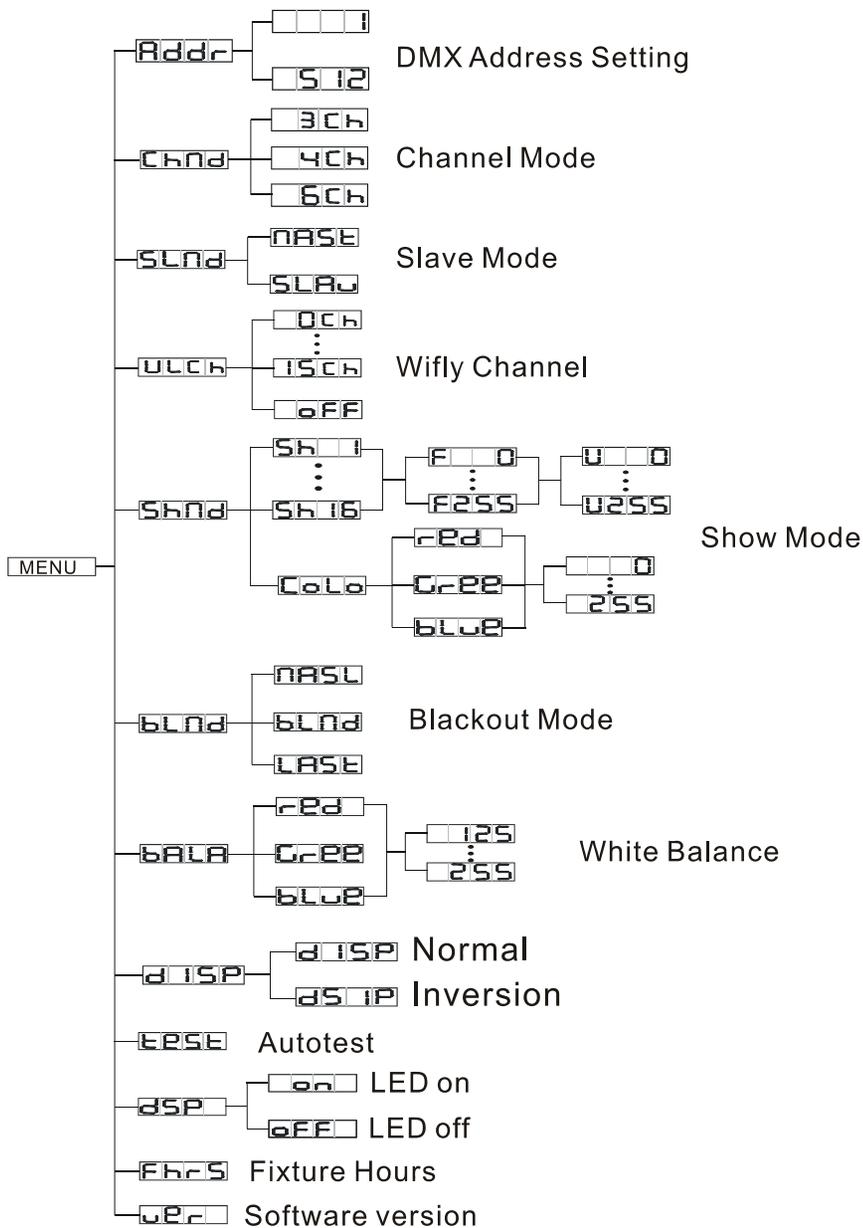
**System Menu:** When making adjustments press **ENTER** to confirm your setup and then press and hold the **MENU** button for at least **3 seconds**. To exit without making any adjustments press the **MENU** button.
