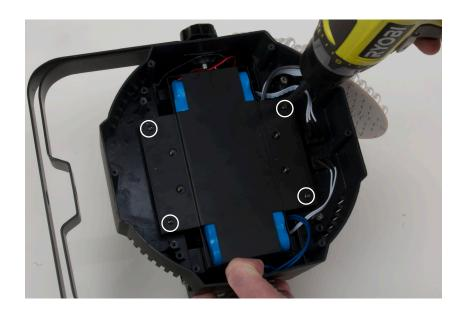
After setting the LED panel to the side, uscrew and remove the 4 phillips screws that hold the battery cover in place.
