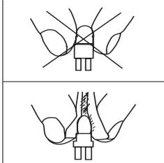
This fixture is fitted with halogen lamps which are highly susceptible to damage if improperly handled. Never touch the lamps with your bare fingers as the oil from your hands will shorten lamp life. Also, never move the fixture until the lamps have had ample time to cool. Remember, lamps are not covered under warranty conditions.
