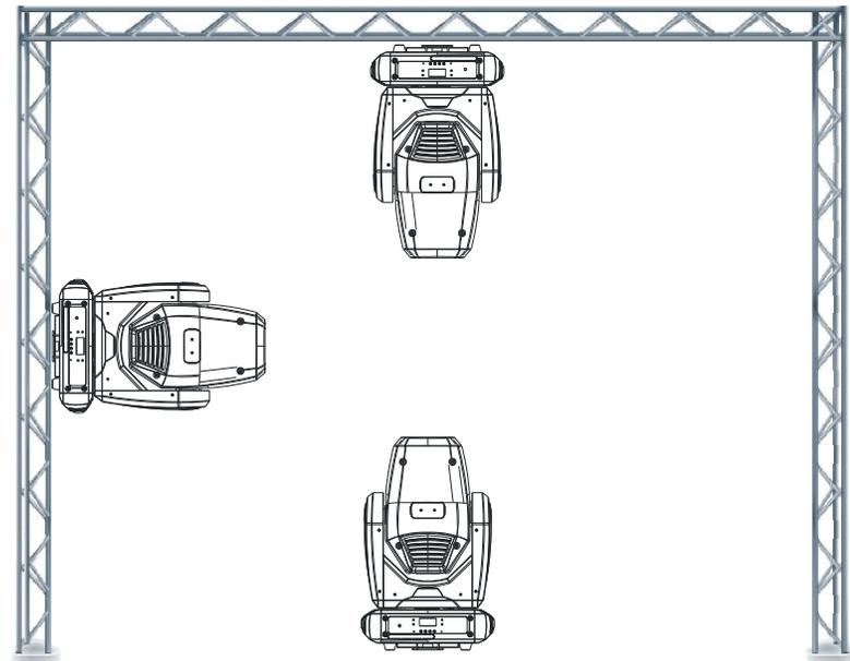
The Focus Spot Three Z is fully operational in three different mounting positions, hanging upside-down from a ceiling, mounted sideways on trussing, or set on a flat level surface. Be sure this fixture is kept at least 0.5m away from any flammable materials (decoration etc.). Always use and install the supplied safety cable as a safety measure to prevent accidental damage and/or injury in the event the clamp fails (see next page).
