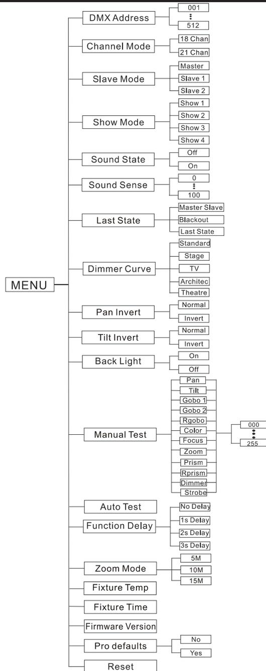
**System Menu:** When making adjustments press **ENTER** to confirm your setup then press and hold the **MENU** button for at least 3 seconds. To exit without making any adjustments press the **MENU** button. The display will lock after 30 seconds, press the **MENU** button for 3 seconds to unlock.
