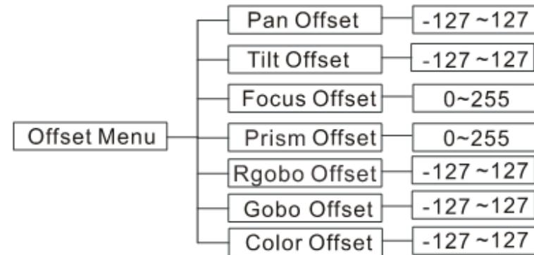
To enter the Offset Menu, press the MENU button to unlock the display, then press the ENTER button for at least 5 seconds. In this sub-menu you are able to adjust the home position of the pan, tilt, focus, prism, rotating gobo motor, gobo wheel, and color wheel. To exit this menu press and hold the MENU button.
