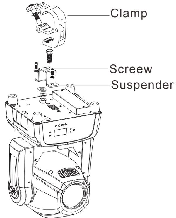
Screw one clamp via a M12 screw and nut to the included bracket. Attach the bracket using the omega locks to the bottom of the Focus Spot Two. Attach and pull the safety-cable through one of the safety holes located on the bottom base and over the trussing system or a safe fixation spot. Insert the end in the carabine and tighten the safety screw.
