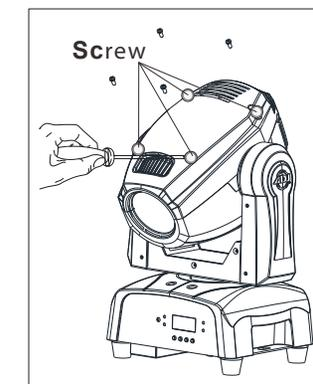
4. Unscrew the 4 screws located on the other side
