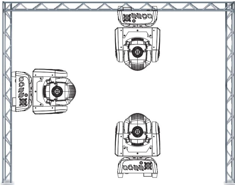
The Focus Spot Two is fully operational in three different positions, hanging upside-down from a ceiling or trussing, mounted sideways on trussing, or set on a flat level surface. Be sure this fixture is kept at least 0.5m away from any flammable materials (decoration etc.). Always use and install the supplied safety cable as a safety measure to prevent accidental damage and/or injury in the event the clamp fails (see next page).
