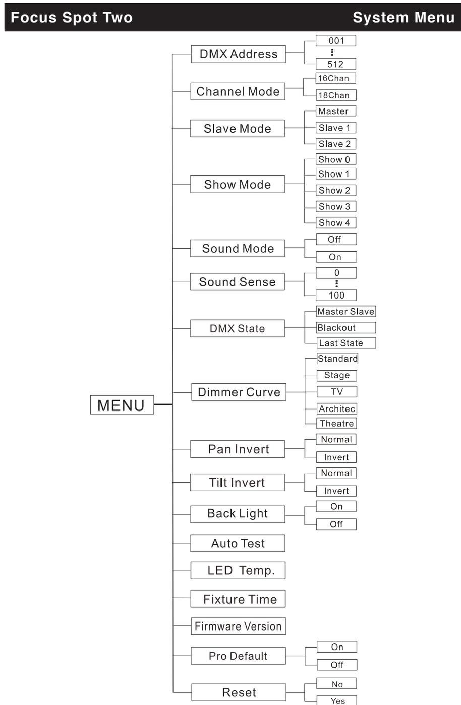
**System Menu: When making adjustments press ENTER to confirm your setup then press and hold the MENU button for at least 3 seconds. To exit without making any adjustments press the MENU button. The display will lock after 30 seconds, press the MENU button for 3 seconds to unlock.**
